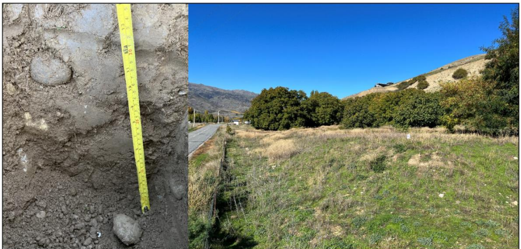
8. Fill with mixed subsoil and stones.
