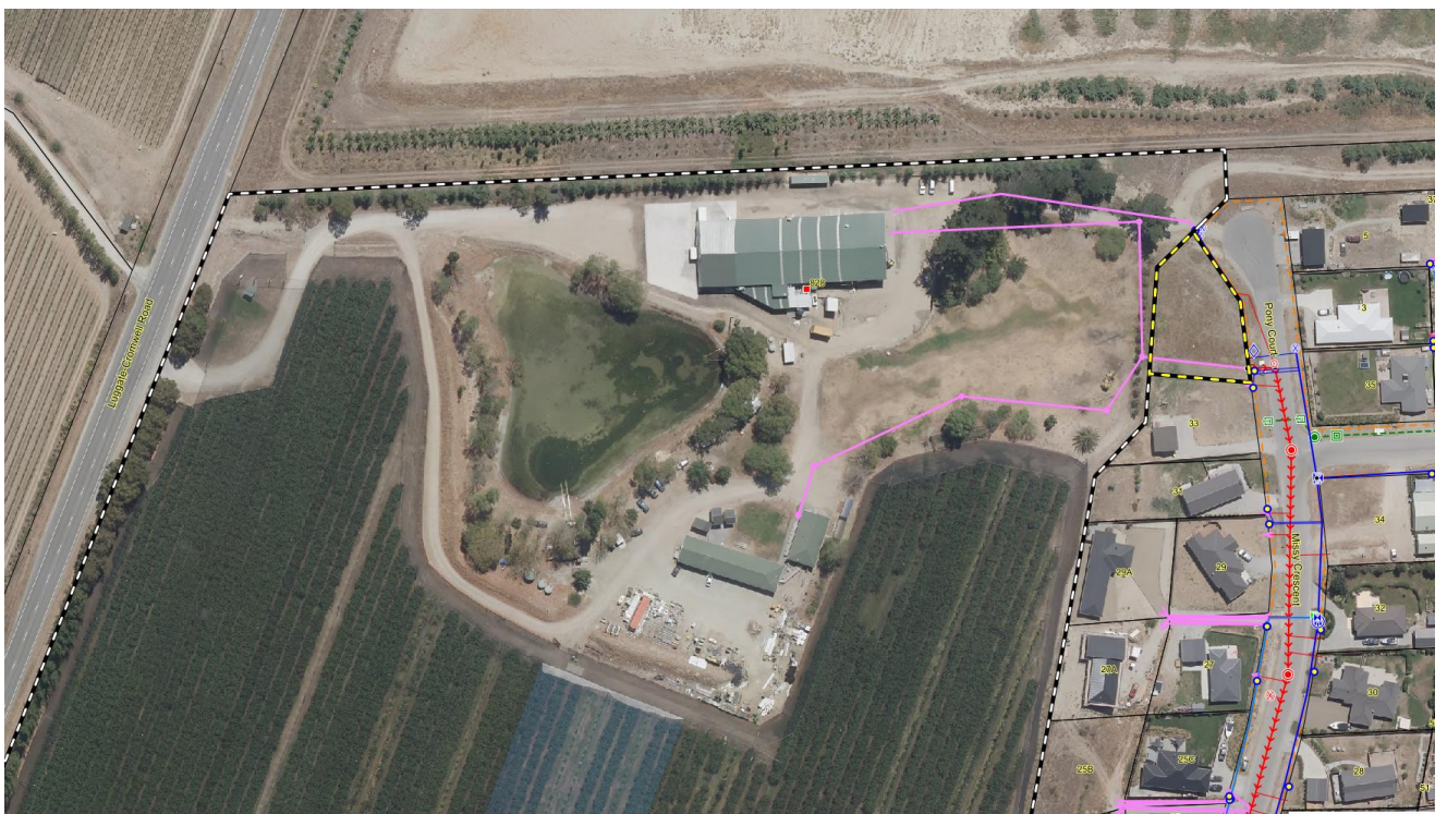
Figure 2: CODC GIS Image 2 (Showing existing water and wastewater services connections off the Council Pisa Village water and wastewater mains in Pony Court, for the existing packhouse and workers accommodation at the northern end of the site)
