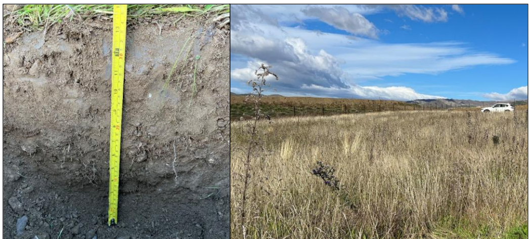
3. Reinstated soil - shallow stony soil with compact mixed topsoil over compact gravel surface.
