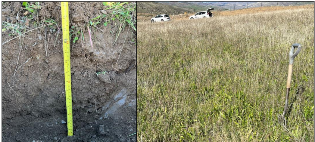
1. Reinstated soil - shallow stony soil with compact mixed topsoil over compact gravel surface.
