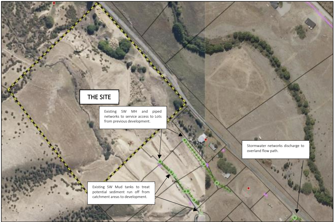
Figure 4 Existing stormwater infrastructure from the adjacent development (image from CODC Intramaps, retrieved on 30-08-2022).
