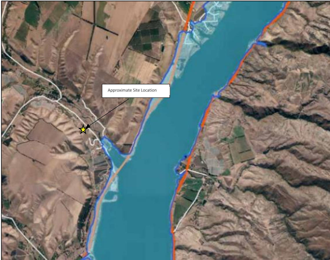
Figure 6. Inundation map based on the Hawea Lake Dam Break Analysis Update Report – 2011 (image from Cromwell Community Response Plan 1 )
