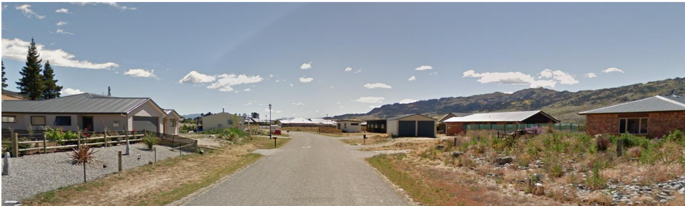
Photograph 9: Typical character of Pisa Moorings streetscape, with no street tree plantings, no footpaths, swale drainage, suburban street lighting and a variable approach to fencing.
