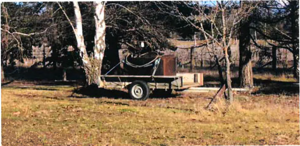
Mobile diesel tank for filling house heating system, next to the existing house.
