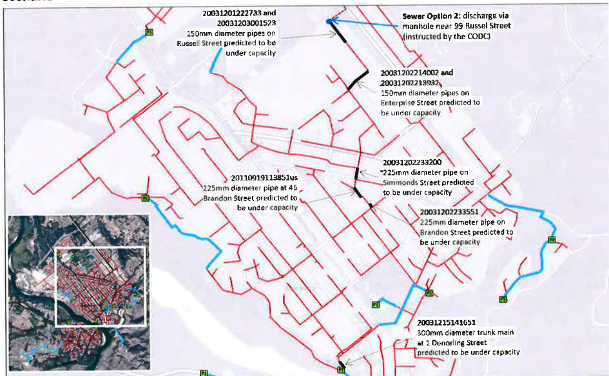
Figure 4.2: Location of additional pipes under capacity and overflows in Option 2 Plan Change WWF scenario
