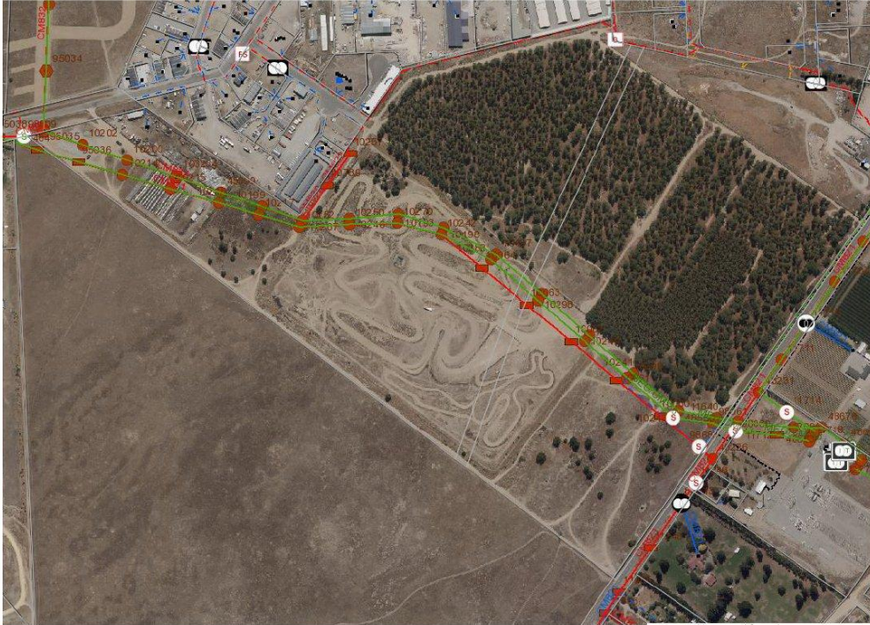
Figure 1 - Aurora Energy Lines and support infrastructure crossing the proposed IRA extension
