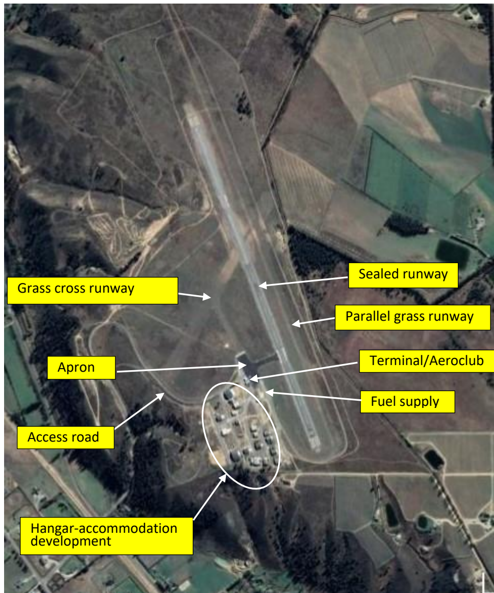
Figure 3: Operational areas and hangars-accommodation
