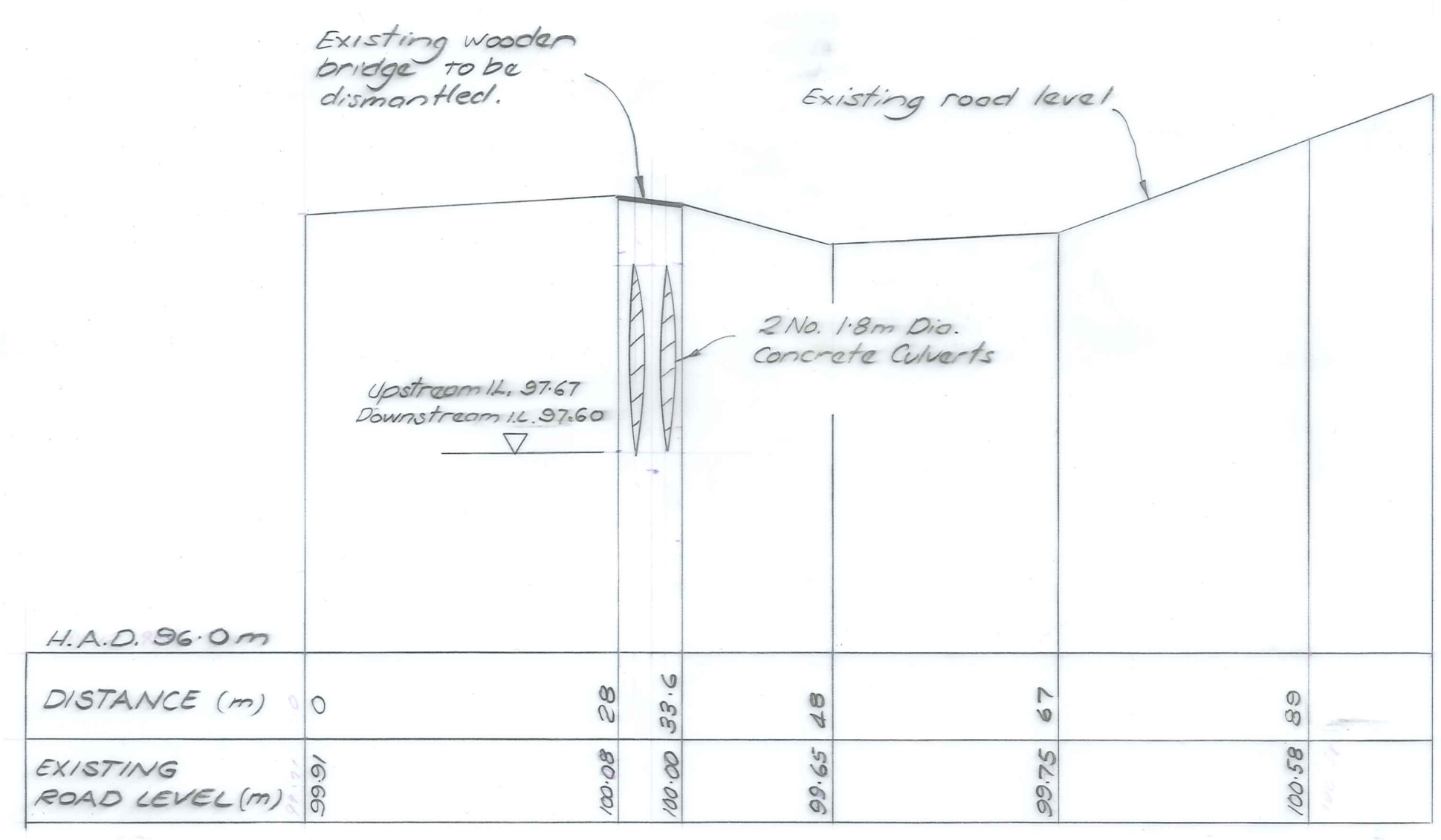
LONGITUDINAL SECTION - EXISTING ROAD Scale Horiz. 1:1000 Vert. 1:100
