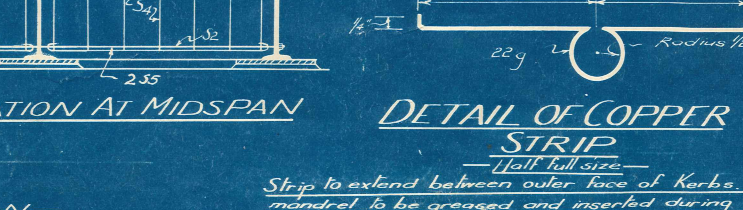
DETAIL OF COPPER STRIP Full full size Strip to extend between outer face of kerbs, 1" mandrel to be greased and inserted during concreting and be withdrawn while concrete is still green - 14 off.
