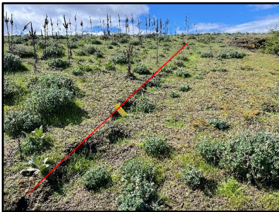
Photo 3: Image showing slope displacement on crest of bank in Lot 9.
