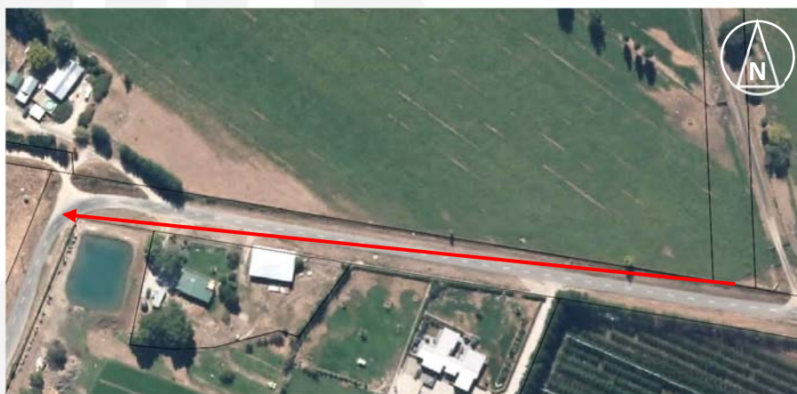
Figure 8: Sight Distance Towards the West at the Proposed Site Access
