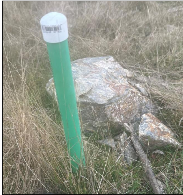
Figure 12 Photo of piezometer (source; HML).
