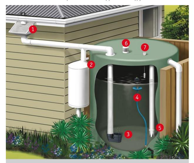
**Debris Diverter** Prevents leaves and debris from entering the downpipe.
