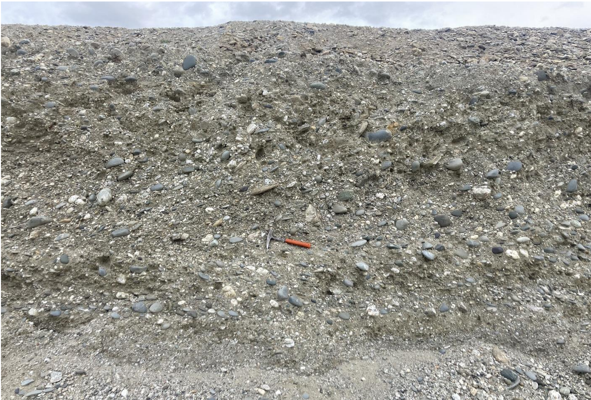
Photo 2. Outwash gravel exposed in a bench cut within the test pit. This particular face is 4 m high and cut sub-vertically. Geological hammer for scale in the centre of image.
