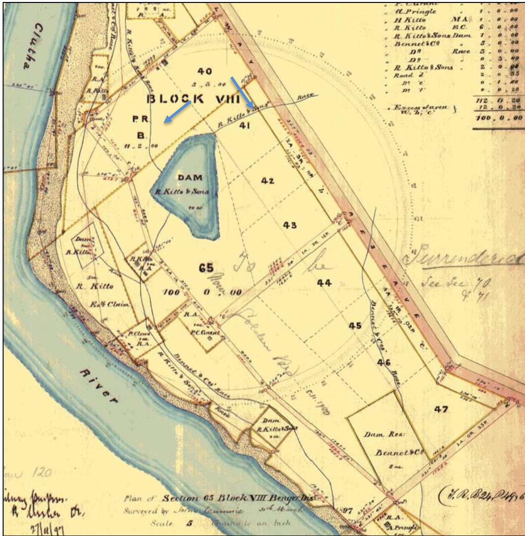
Figure 2. Detail of S03225, dating to 1897, showing water races identified in the site survey (blue arrows).
