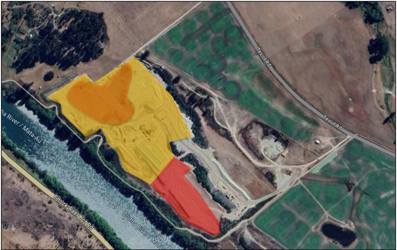
Figure 1-4. Aerial imagery showing prior exploration works undertaken by Hawkeswood Mining Limited Under Exploration Permit 60712 showing area excavated to approximately 1.5m (highlighted yellow); 16m (highlighted orange); and between 200-300mm (highlighted red).
