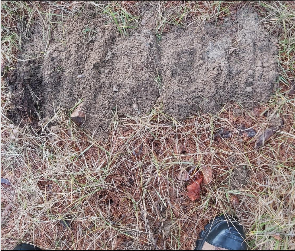
Photograph 2 Hand Auger 5 indicates Category 1 soils encountered directly below topsoil.
